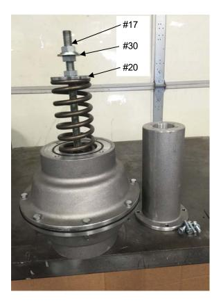
Pay particular attention to the assembly of jamb nuts and washers at the upper end of the Spring Rod (item 17).
