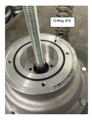
The actuator has been inverted and the stem (item #5) is now projecting upward from the bottom of the actuator.
