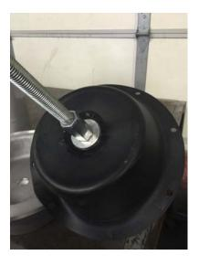
Gently remove the stem and diaphragm plate / diaphragm assembly and turn it upward.
