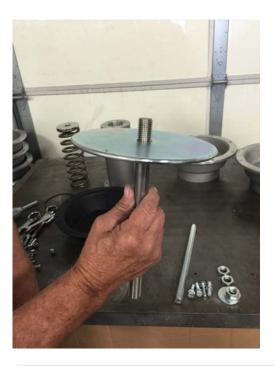
Lay new replacement diaphragm over diaphragm plate w/top of stem projecting up through center hole of replacement diaphragm.
